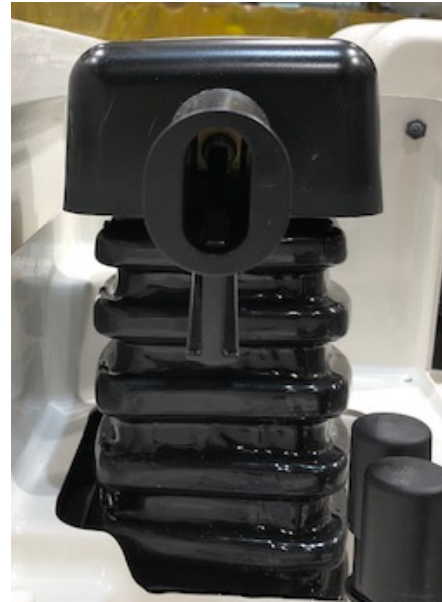
FIGURE 11 - Example of a properly adjusted single stick controller
