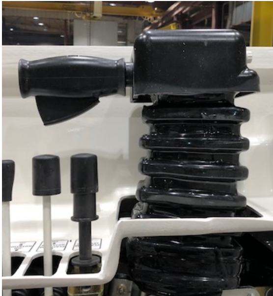
FIGURE 11 - Example of a properly adjusted single stick controller
