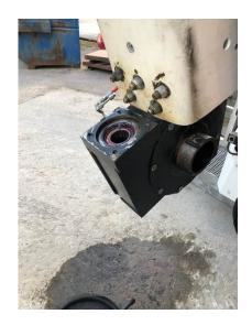
Place a drip pan below the gear box and remove the cover plate. Use a sharp chisel to help pry the cover plate off.
