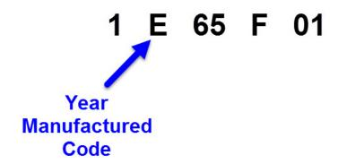
Use the chart below to determine the year based on the code provided. In this example the unit was manufactured in 1990.
